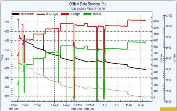
The tool calculates **multiphase rates** using dP in the wellbore using a **direct numerical integration** to the Mechanical Energy Balance and **rigorous PVT**
