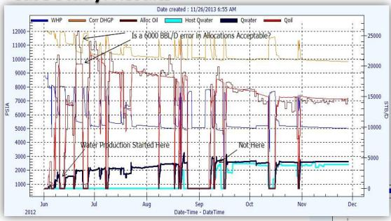
As it turned out, the water production started from the day the well was brought online. The operator's allocations were off up to 6,000 BBL/D
