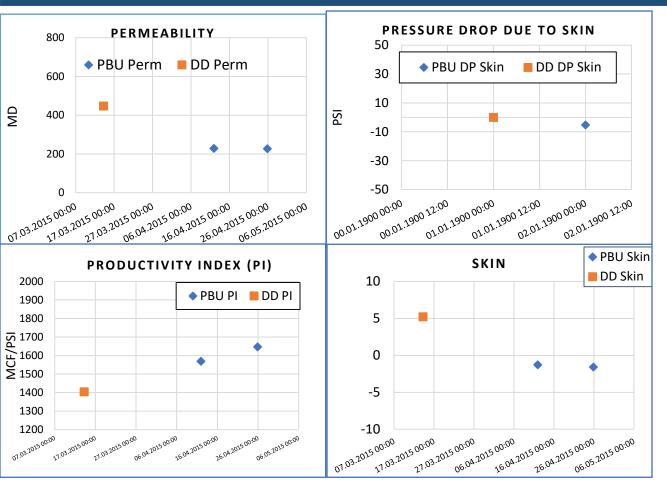
Each PBU and DD test are analyzed for diagnostic PTA parameters in real-time
