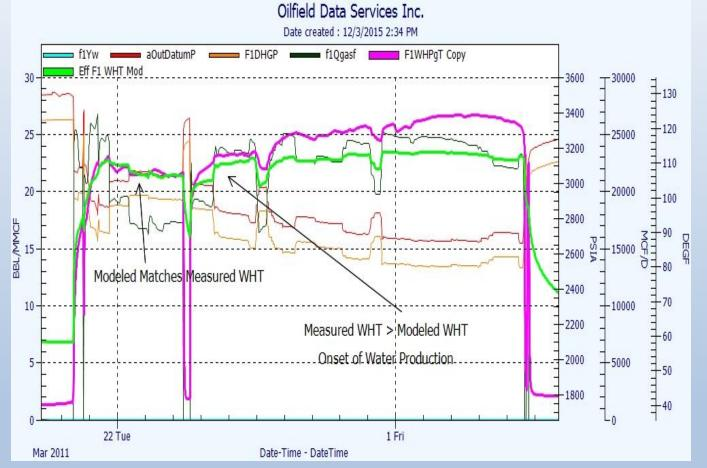
The function in purple is the measured wellhead temperature. Notice the sudden increase in the measured temperature and departure from the modeled temperature
