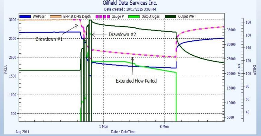
The dynamic response of the well for single-phase conditions (or for known composition of entrained fluids) needs to be calibrated using a multi-rate test
