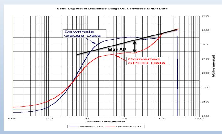
The maximum pressure difference between the measured data before and after reinjection occurs can be used to calculate the water yield after the onset of water production
