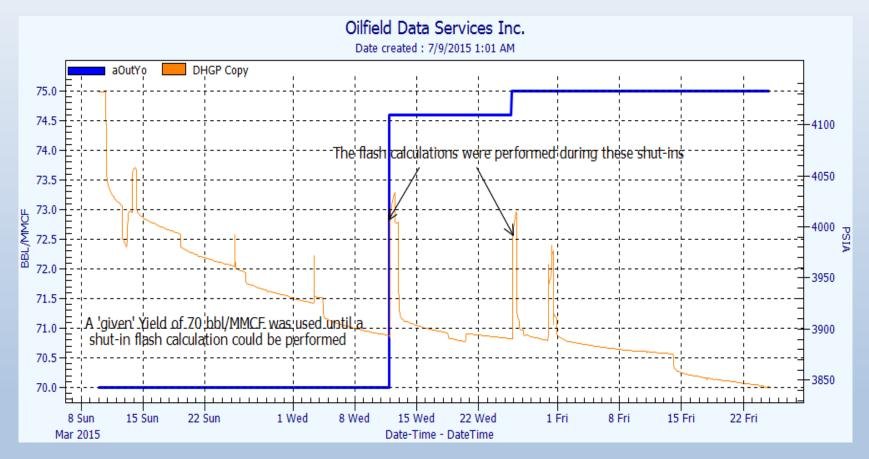
A 'flash' calculation can be performed automatically after the well is shut-in. The liquid yield can be calculated during every shut-in and can then be used as an input for the pressure and rate calculations
